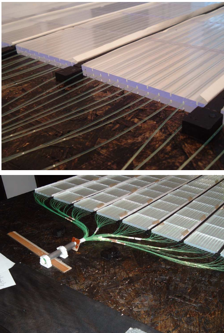
Fig. 1. WLS fibres in the scintillating tiles and assembling the detector.
